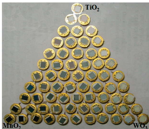
Figure 3. Photograph of the 66 devices being prepared for high-throughput screening.
